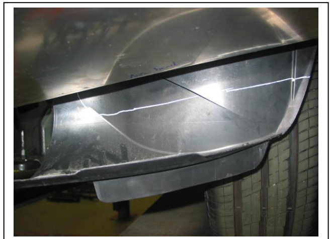
Figure 16: Mark and trim guard liner to fit rear of underbelly guard.
