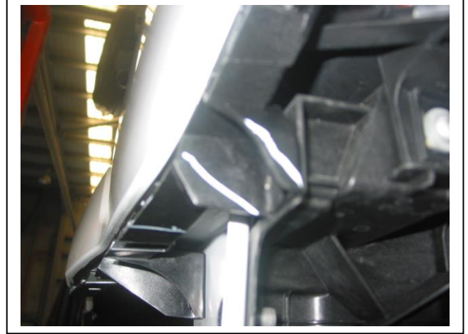
Figure 2: Trim locator to suit bumper cut
