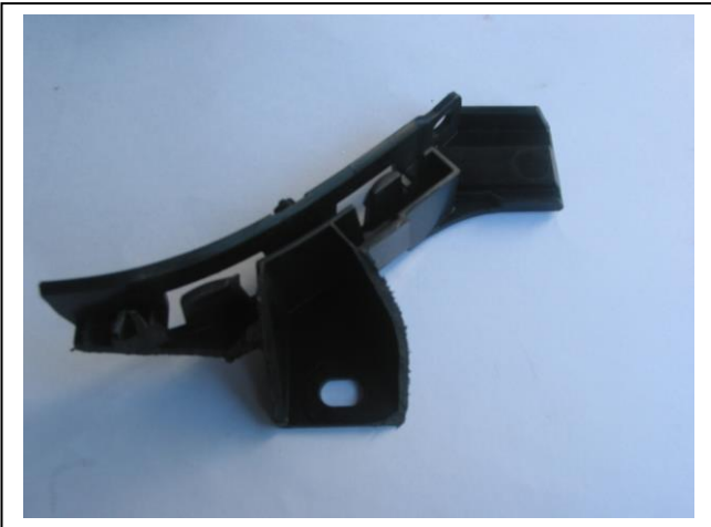
Figure 3: Trimmed locator after cut
